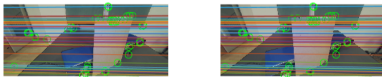
Figure 1: Rectified Stereo Image with parallel epipolar lines
